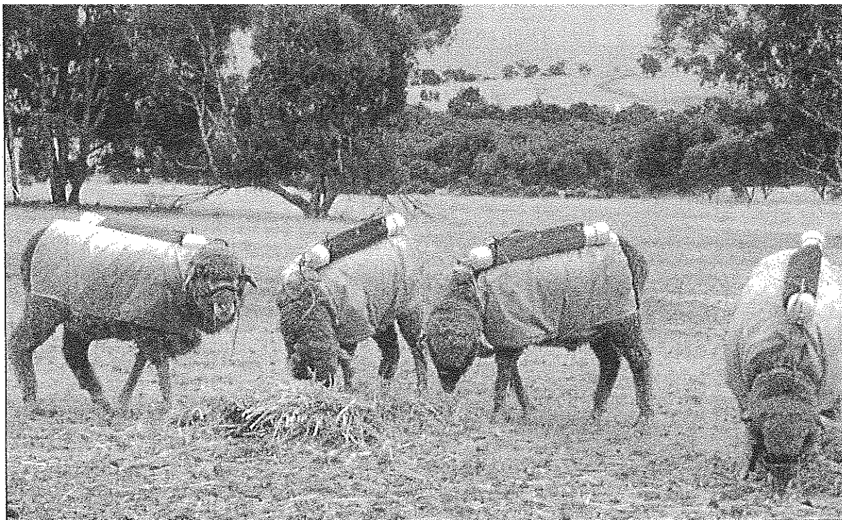
GAS MASKS: Special backpacks collect and record the volume of methane emissions from sheep.
